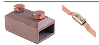
**Oblong Test Clamps** are designed to join conductor tape to facilitate in the annual testing of the Lightning Protection System. The clamp is designed to allow the conductor to be overlapped and secured using bolts. Suitable for use with PVC covered tape.
