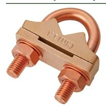
Rod To Tape Type Clamps (U Bolt Double Plate Type) join 25 x 3 conductor tape to the earth electrode/rebar without the need to drill the tape. The clamps have a high resistance to corrosion and are mechanically strong to ensure a lasting connection.
