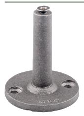
**Back Plate holdfast** maintains a set distance of 75mm between lightning conductor and the surface of the structure being protected (when required).
