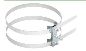
The **Double Pipe/Handrail Bracket** is manufactured from stainless steel and is used in conjunction with **Cable Holders** having an M8 or M16 threaded insert and **Mast Holders** having M16 threaded inserts.
