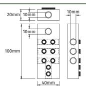
For connecting several Insulated Lightning Conductor cables together at the end of the cable run.
