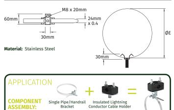
Single Pipe/Handrail Bracket with M8 fixings are used in conjunction with Insulated Lightning Conductor Cable Holders having an M8 threaded insert.
