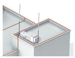
When used in conjunction with Kingsmill Insulated Lightning Conductor cable, the Air Terminal can be placed closer to objects that require protection. The cable simulates a separation distance of ≤0.75m in air and ≥1.5m in solid material.
