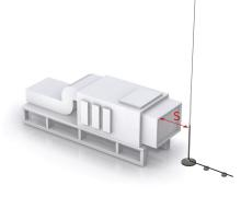
Used where there is sufficient roof space to maintain the appropriate separation distance between the mast and the object being protected.
