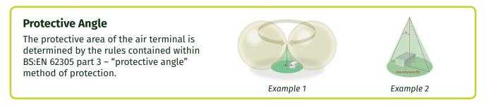
The minimum separation distance between the object being protected and the Lightning Protection System, is calculated according to the formulae for separation distances, given in BS:EN 62305 part 3.
