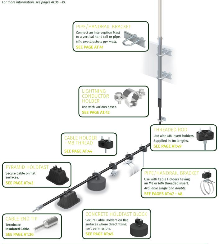
Figure AT:6 - Example of an Insulated Lightning Conductor Cable installation showing various accessories
