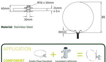
COMPONENT Single Pipe/Handrail Insulated Lightning ASSEMBLY: Bracket Conductor Mast
