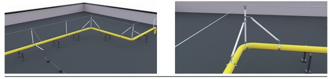
Figure AT:7 - Isolation bars used to protect a pipeline
