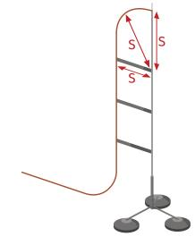
Maintains separation distance using **Insulated Separation Bars**.
