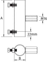
The **Air Terminal Mast Holders with Threaded Insert** are designed for use with our insulated and steel/insulated Air Terminal Masts.
