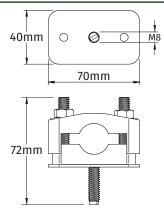
The **Insulated Lightning Conductor Cable Holder** is supplied with an M8 threaded stud.
