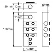
For connecting several Insulated Lightning Conductor cables together at the end of the cable run. Used outside the separation distance area.
