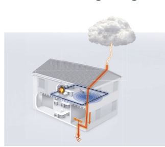
Inductive coupling - electro-magnetic field from a direct strike
