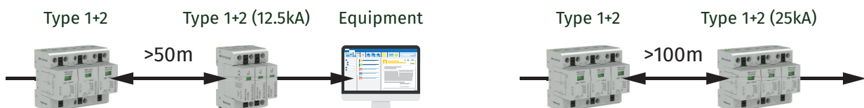
Figure SPD:10. Type 1+2 devices protective distances
