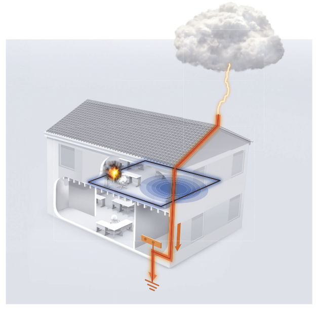
Figure SPD:3. Inductive Coupling - Example 1 (induced electro-magnetic field)
